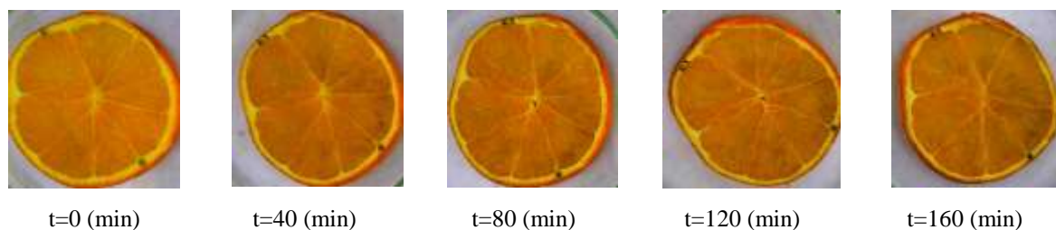
Fig. 3. The sample images during drying process for thickness 0.5 mm
