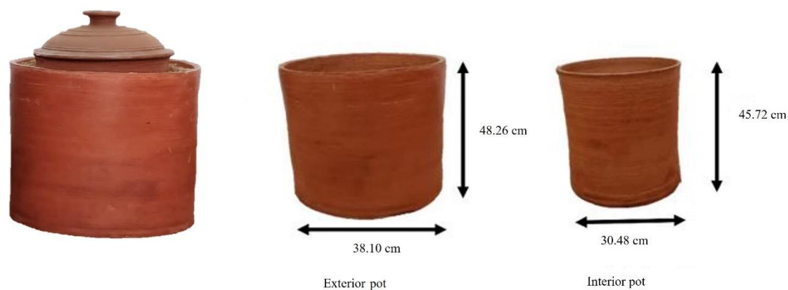
Fig. 2. The details of the clay pot cooler.
